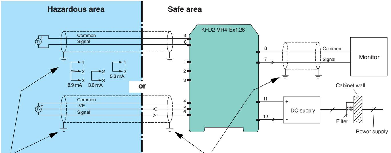
If the transducer and probe are isolated from ground, the cable screen may be left unconnected at this end but must be securely insulated. If the transducer circuitry is connected or decoupled to ground the screen must be securely grounded.
