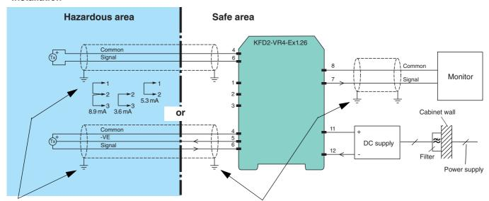
If the transducer and probe are isolated from ground, the cable screen may be left unconnected at this end but must be securely insulated. If the transducer circuitry is connected or decoupled to ground the screen must be securely grounded.
