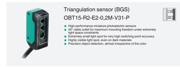
Triangulation sensor with background suppression for standard applications, miniature design, 15 mm detection range, red light, light on, PNP output, 200 mm fixed cable with plug M8, 4-pin
