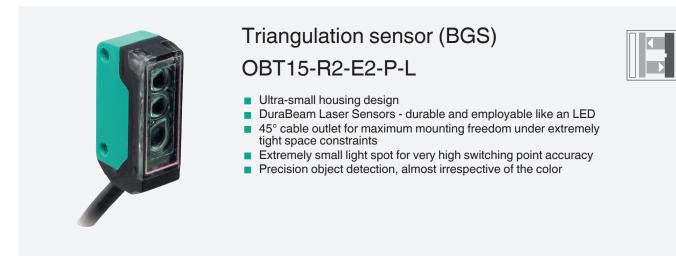
Laser triangulation sensor with background suppression, ultra-small design with M2 mounting, 15 mm sensing range, light on, PNP output, 2 m fixed cable
