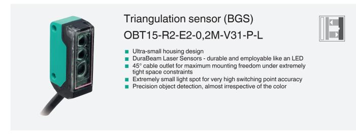
Laser triangulation sensor with background suppression, ultra-small design with M2 mounting, 15 mm sensing range, light on, PNP output, 200 mm fixed cable with plug M8, 4-pin
