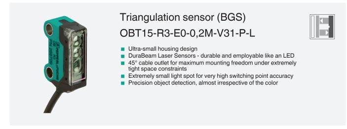
Laser triangulation sensor with background suppression, ultra-small design with M3 mounting, 15 mm sensing range, light on, NPN output, 200 mm fixed cable with plug M8, 4-pin
