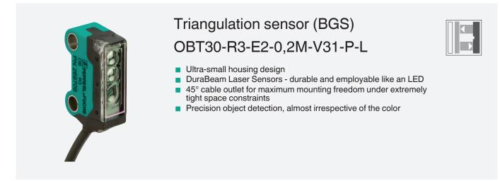
Laser triangulation sensor with background suppression, ultra-small design with M3 mounting, 30 mm sensing range, light on, PNP output, 200 mm fixed cable with plug M8, 4-pin
