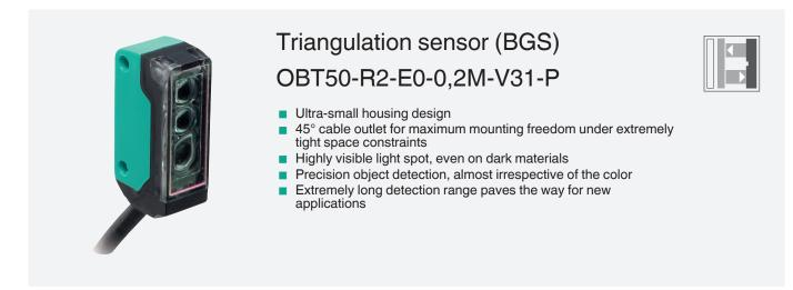
Triangulation sensor with background suppression for standard applications, miniature design, 50 mm detection range, red light, light on, NPN output, 200 mm fixed cable with plug M8, 4-pin
