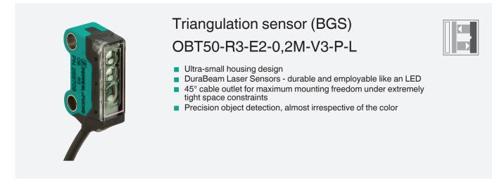
Laser triangulation sensor with background suppression, ultra-small design with M3 mounting, 50 mm sensing range, light on, PNP output, 200 mm fixed cable with plug M8, 3-pin
