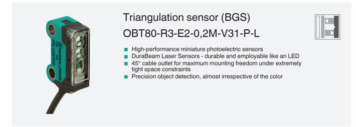
Laser triangulation sensor with background suppression, ultra-small design with M3 mounting, 80 mm sensing range, light on, PNP output, 200 mm fixed cable with plug M8, 4-pin
