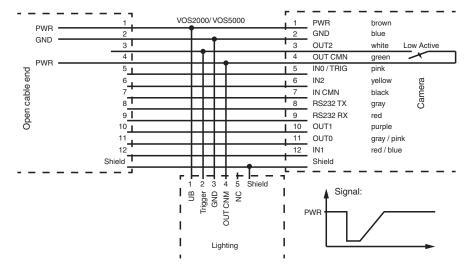
NOTE: With trigger parameterization by means of software, the electrical status of the trigger is output to the outside at GPO2 (OUT2).
