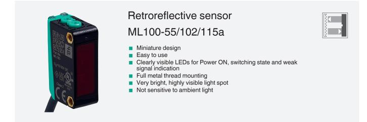
Retroreflective sensor with polarization filter, plastic housing, 5 m detection range, red light, sensitivity adjuster, light/dark on, DC version, NPN output, fixed cable with M8 plug
