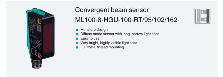
Convergent mode sensor, 100 mm adjustable detection range, red light, light/dark on, NPN output, M8 plug
