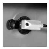
Holding the bracket by the tab, rotate the sensor  $90^{\circ}$  clockwise.
