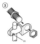
Fasten the two parts of the mounting clamp (a) loosely by means of the screw (b) and the nut (c) supplied.
