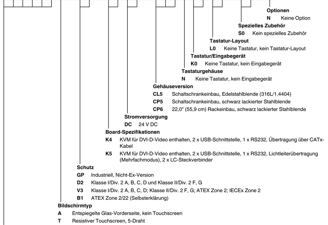
**KM8222** KVM-Monitor, 22,0" (55,9 cm), WSXGA (1680 x 1050 Pixel), KVM angeschlossen
