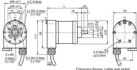
Clamping flange, cable exit radial
