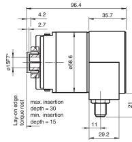
\* shaft can be reduced to ø10F7 or ø12F7 by using an adapter
